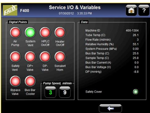
**Figure 71** I/O & Variable Screen
