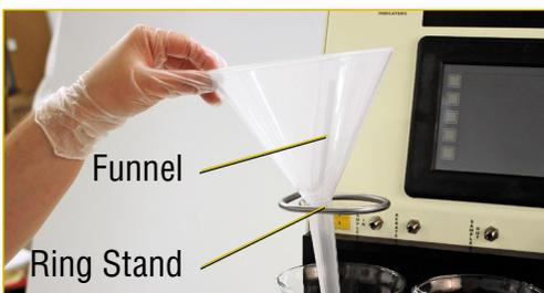
Figure 12 Funnel/Filter Setup
