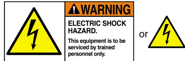
**ELECTRICAL SHOCK HAZARD:** This symbol indicates hazardous voltage is present when opening the electrical cabinet. This unit is to be serviced by trained personnel only.
