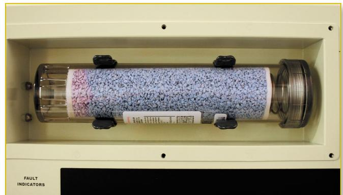
Figure 54 Desiccant Cartridge Mounted In Housing
