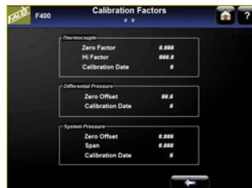
**Figure 69 Calibration Factors Screen**
