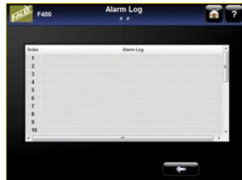
**Figure 72** Listing of most current alarms
