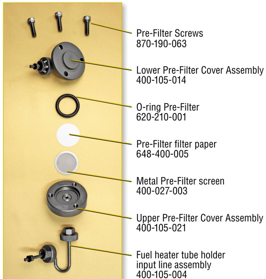
**Figure 8** Components For Assembly of Prefilter
