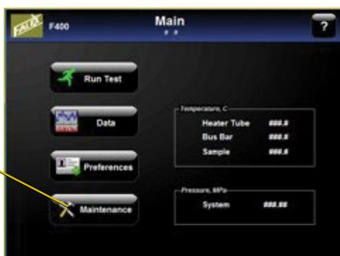
**Figure 57** Accessing The Maintenance Screen
