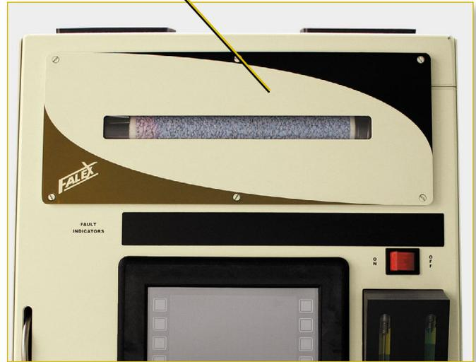
Figure 53 Desiccant Cartridge Location
