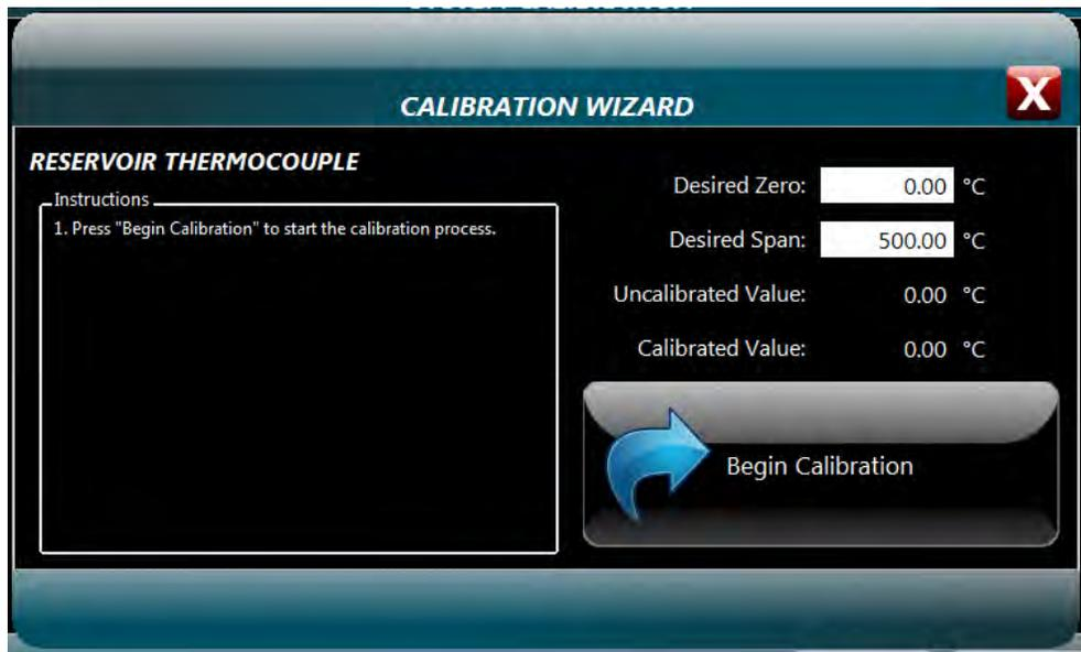
Figure 5-3 – Thermocouple Electronic Calibration Wizard display with Begin button
