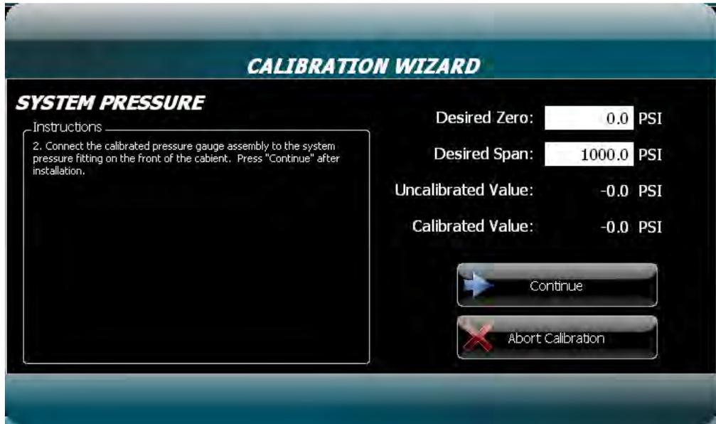
Figure 5-8 – Pressure Calibration Wizard display
