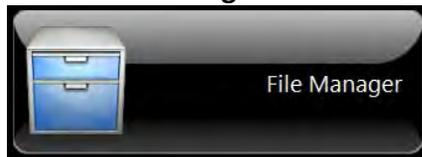
The 'File Manager' selection allows the operator to copy various data files to an external device or delete them from the system (figure 4-72).
