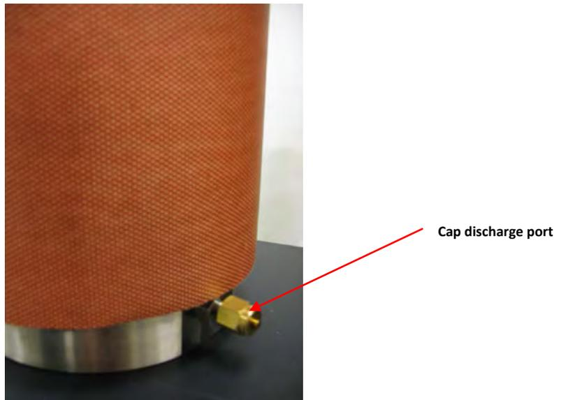
Figure H13 – Cap reservoir #2 discharge port
