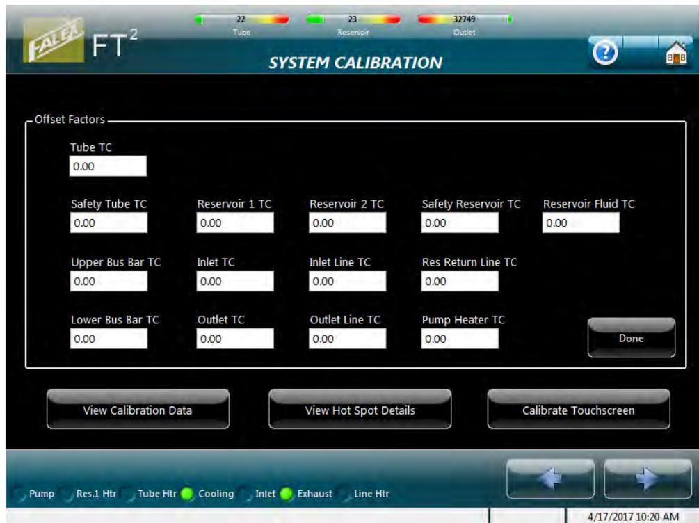
Figure 4-79 – Thermocouple Offset Factor display
