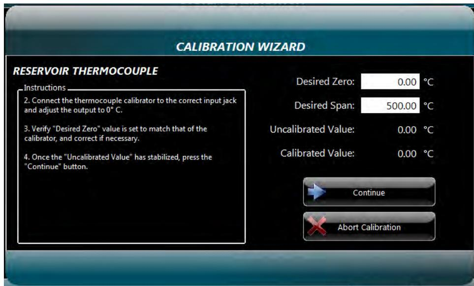
Figure 5-4 – Thermocouple Calibration Wizard display
