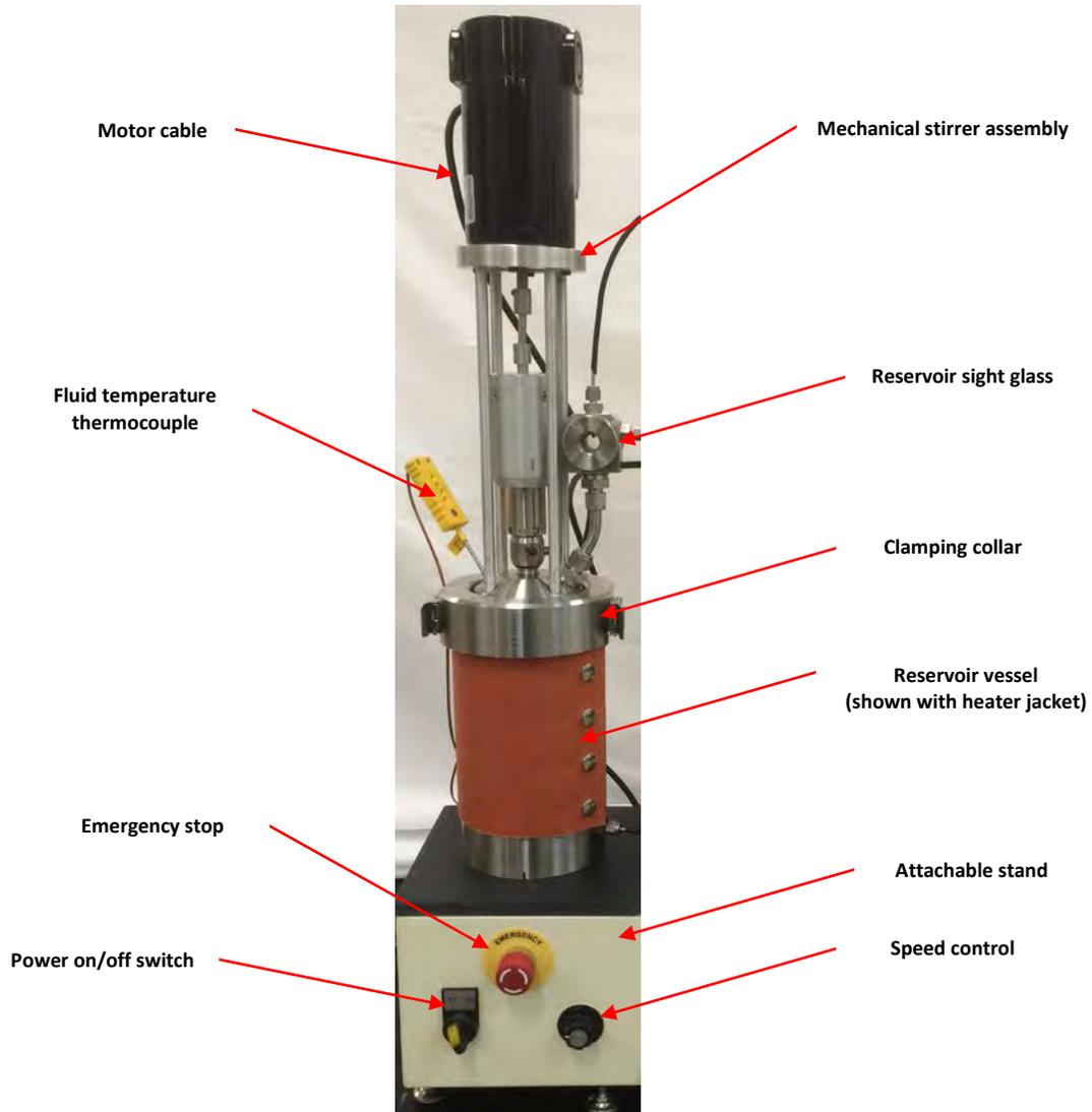
Figure J1 – Mechanical stirrer assembly
