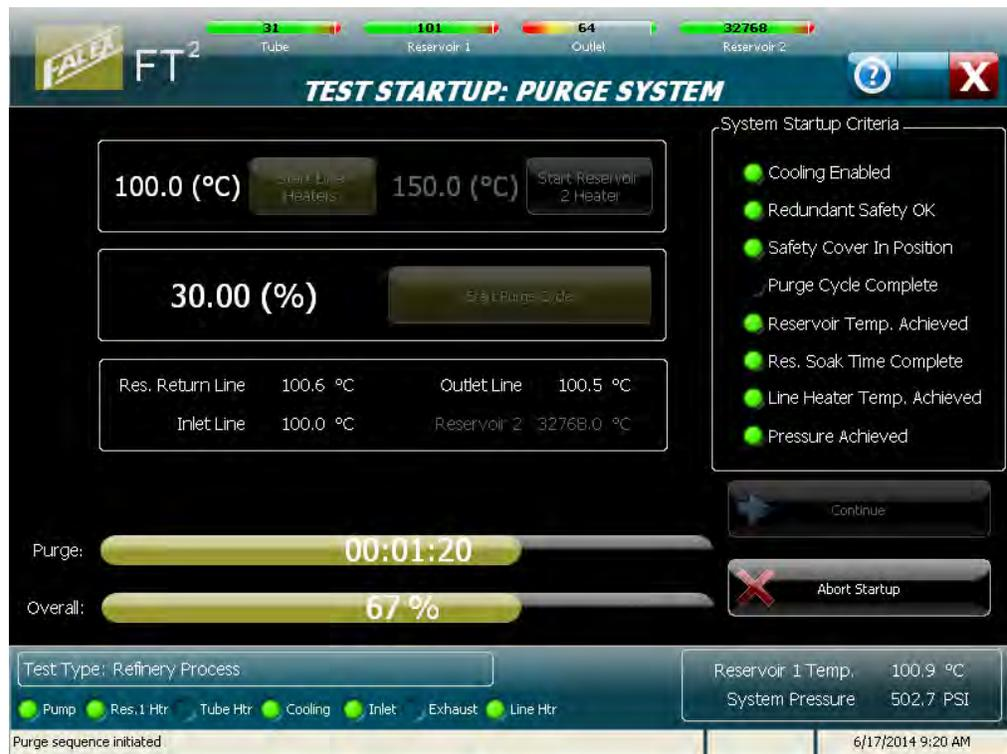
Figure 4-33 – Purge System display (with purge already initiated and line heaters enabled and already initiated)
