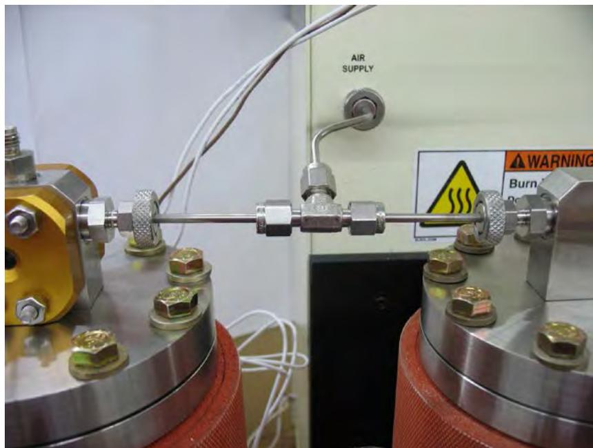
Figure H8 – Pressurization line assembly connection
