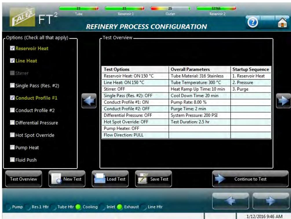
Figure 4-24 – Refinery Process test configuration (summary)
