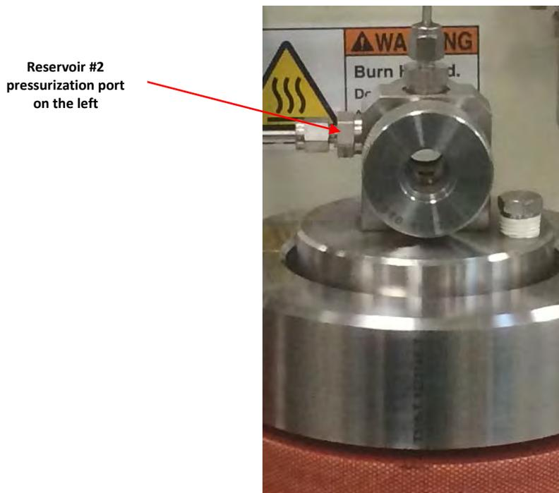
Figure H14 – Reservoir #2 top orientation
