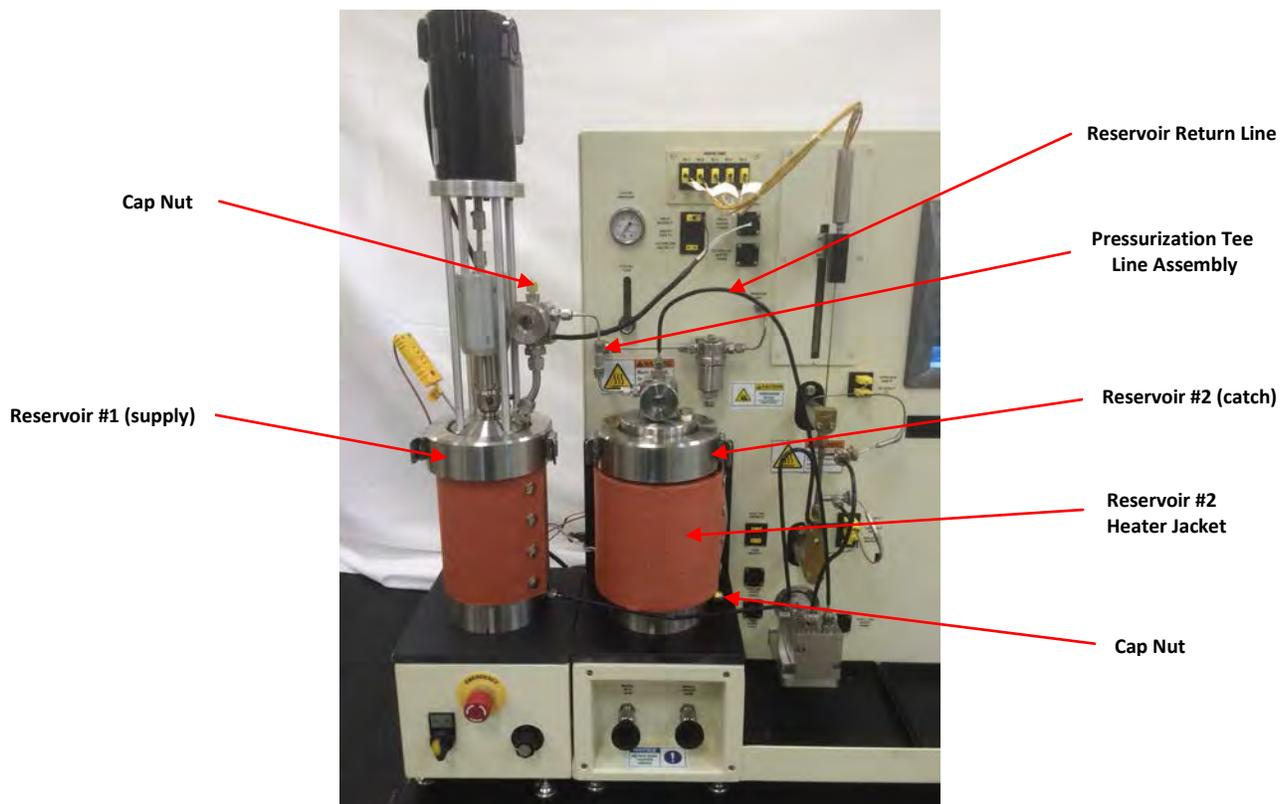
Figure H11 – Single Pass (2<sup>nd</sup> reservoir)
