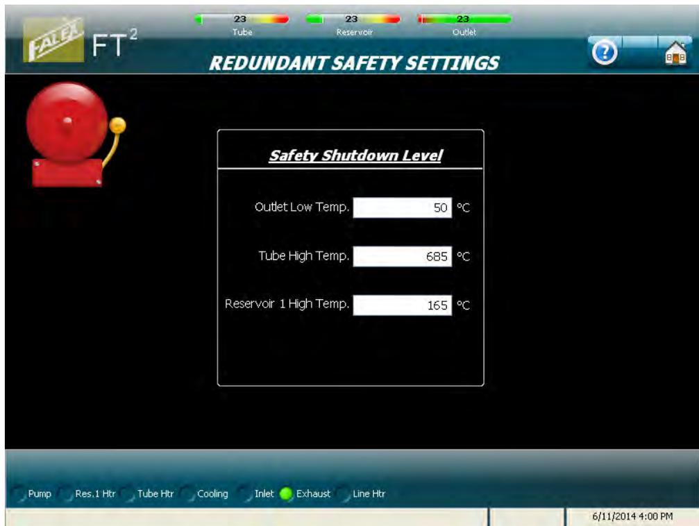
Figure 4-65 – Redundant Safety display (standard)
