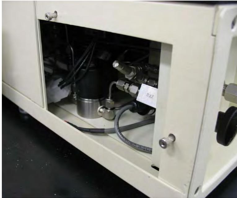
Figure J3 – Shoulder screws installation
