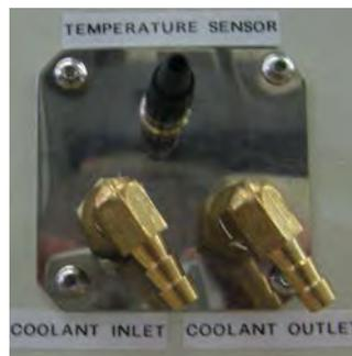
Figure 2-3 – FT<sup>2</sup> External Cooler Connections
