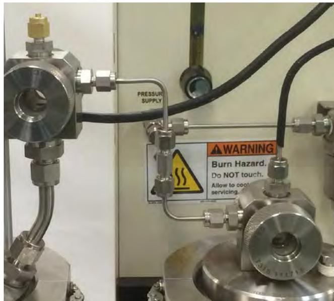
Figure H16 – Pressurization line assembly connection
