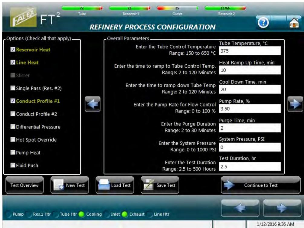
Figure 4-21 – Refinery Process test configuration (standard parameters)
