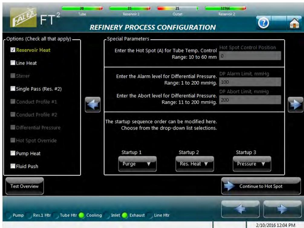
Figure 4-52 – Refinery Process hot spot determination test configuration (special parameter/sequence order)
