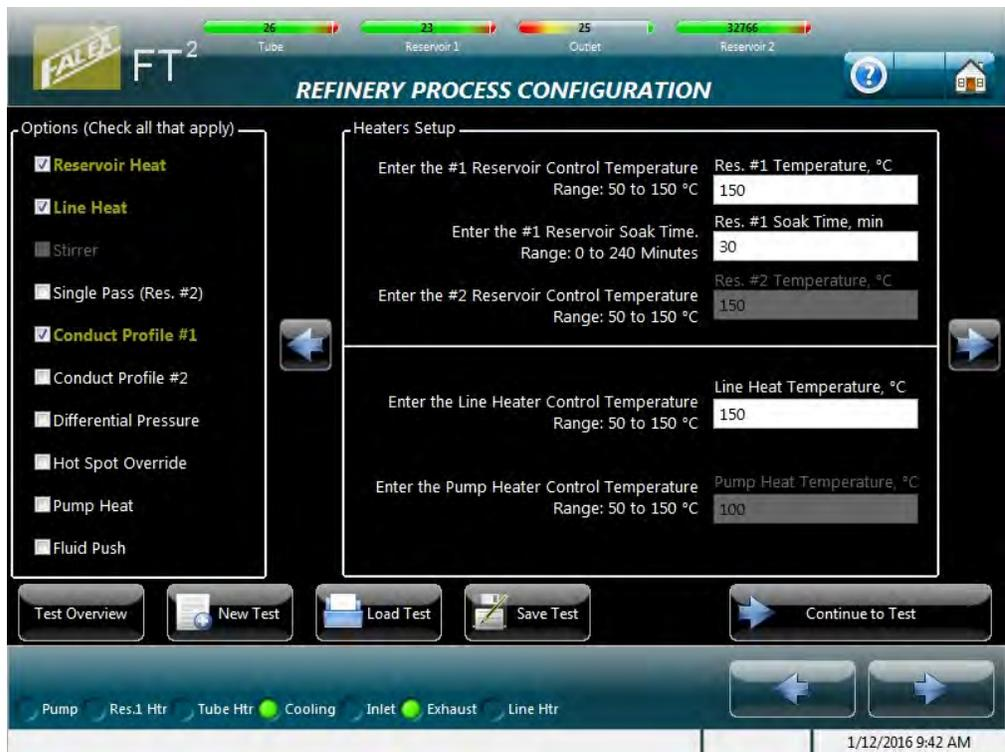
Figure 4-22 – Refinery Process test (optional parameters)
