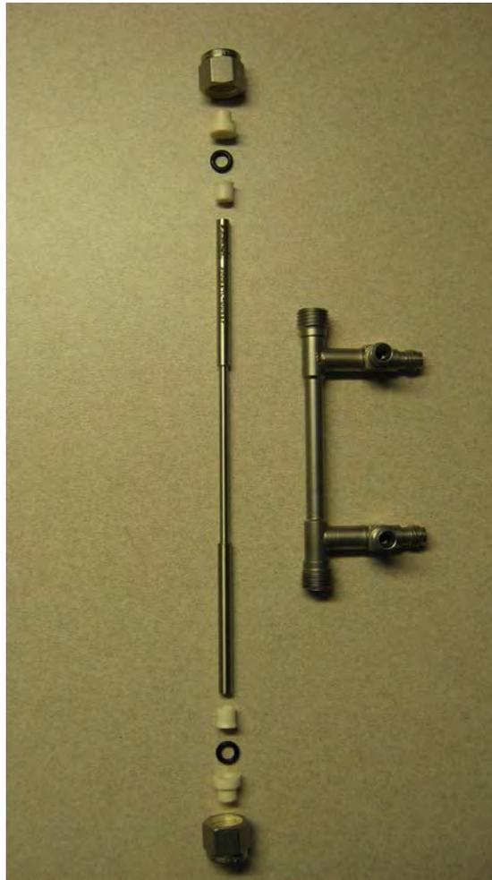
Figure 3-3 – Heater tube holder assembly
