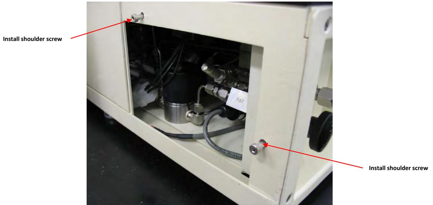
Figure H4 – Shoulder screws installation
