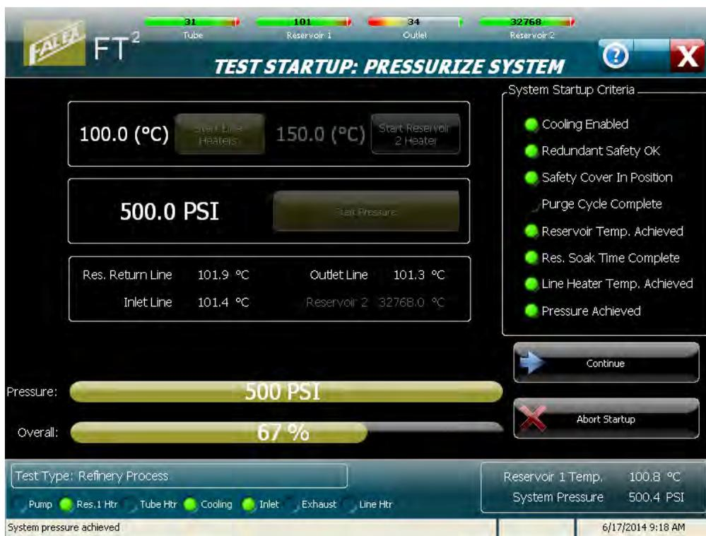
Figure 4-30 – Pressurize System display (with pressurization already initiated and line heaters enabled and already initiated)
