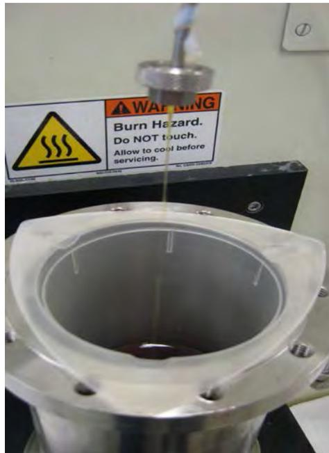
Figure 3-2 – Catch beaker placement
