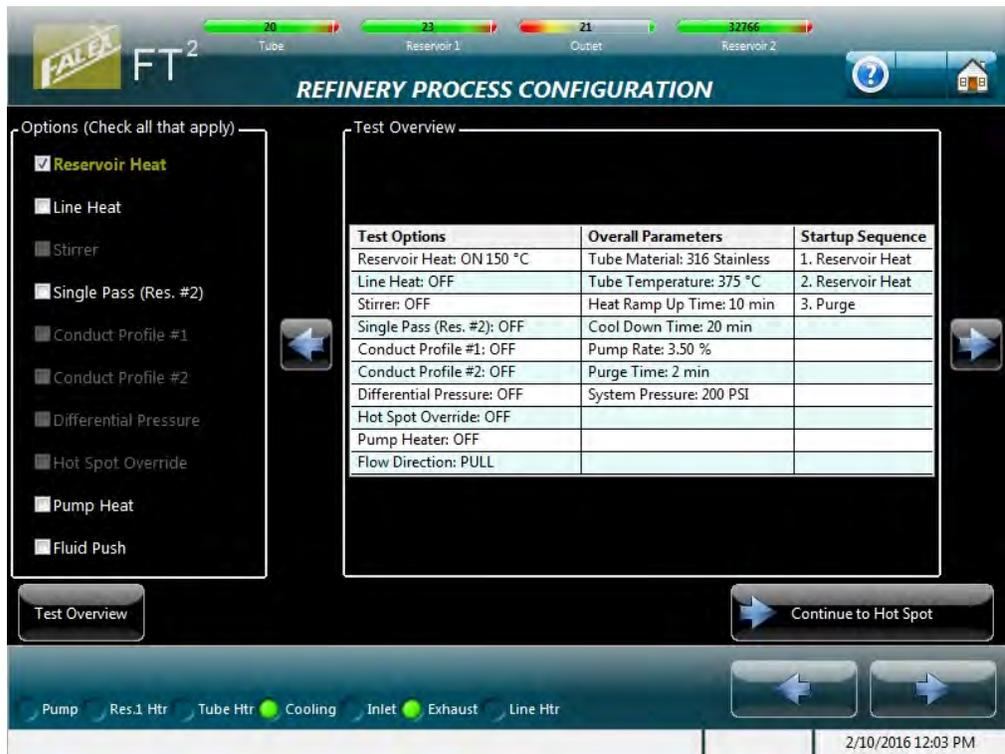
Figure 4-53 – Refinery Process hot spot determination test configuration (summary)
