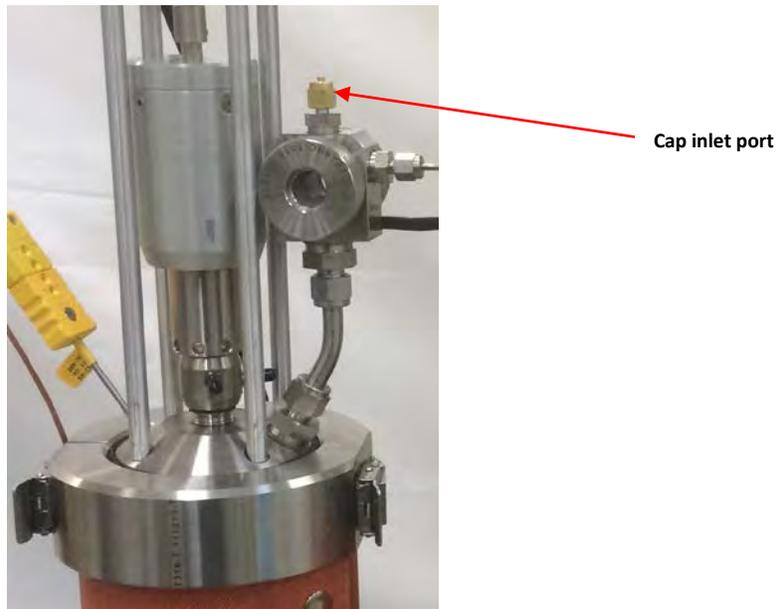
Figure H15 – Cap reservoir #1 inlet port
