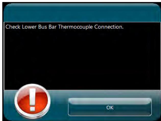
Figure 4-19 – Thermocouple Fail pop-up
