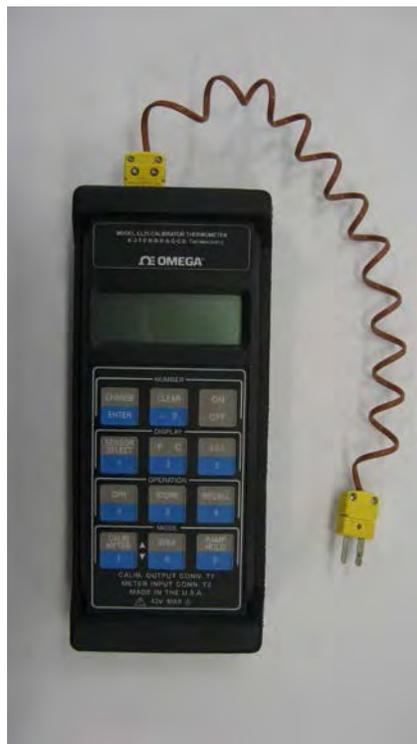
Figure 5-2 – Thermocouple Electronic Calibrator
