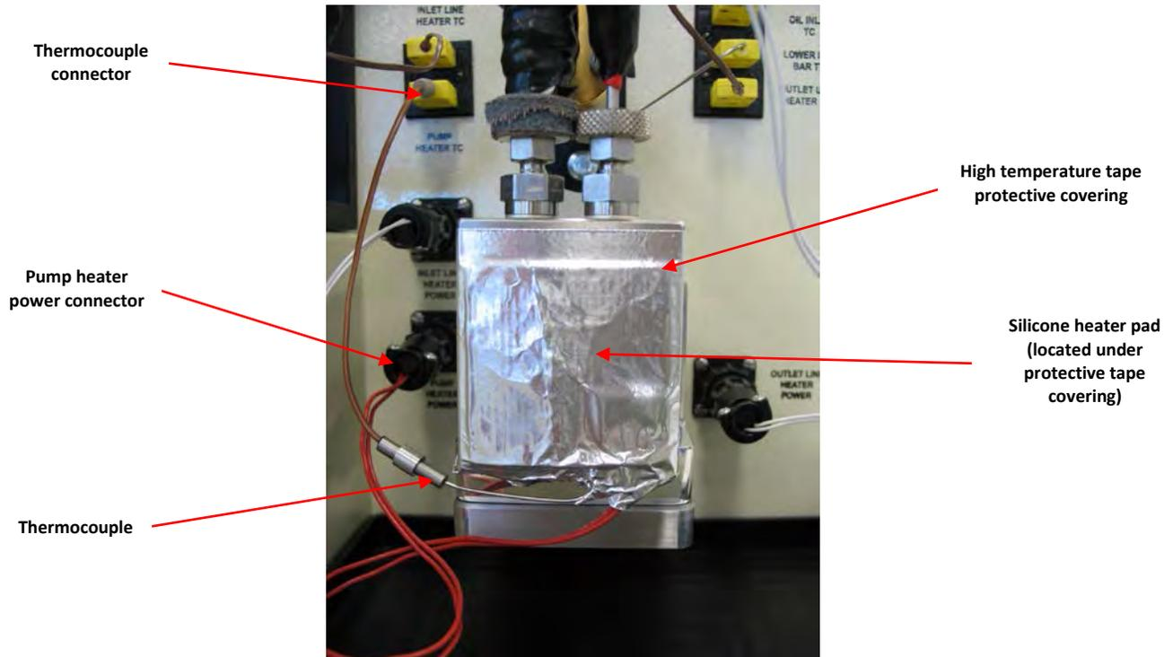
Figure I1 – Pump heater assembly
