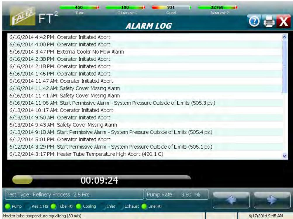
Figure 4-41 – System Alarm Log display
