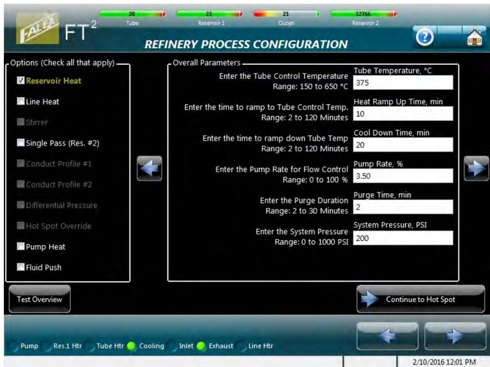
Figure 4-50 – Refinery Process hot spot determination test configuration (standard parameters)
