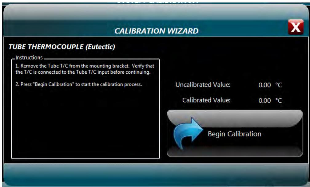
Figure 5-5 – Eutectic Calibration Wizard display with Begin button
