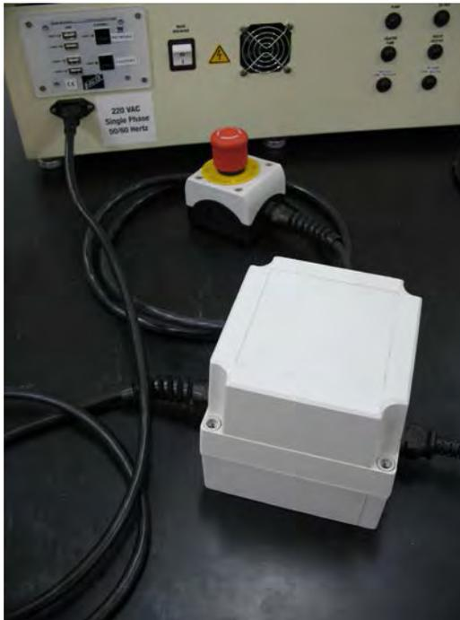
Figure E4 – Installed Remote E-Stop assembly
