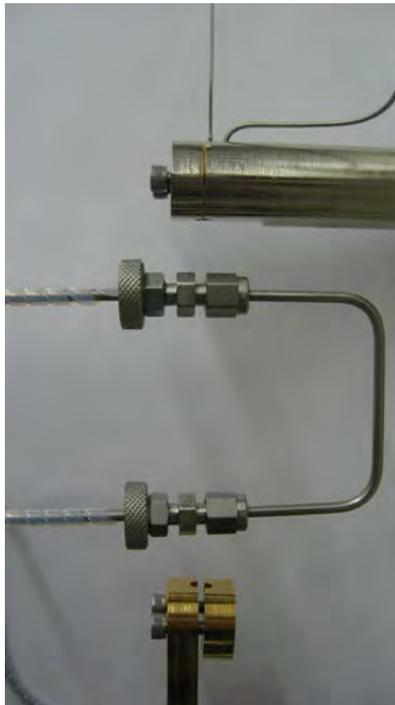
Figure 3-1 – Bypass cleaning line installation
