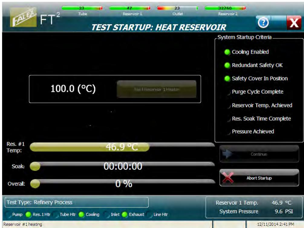
Figure 4-27 – Heat Reservoir display (with heating already initiated)
