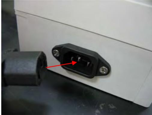
Figure E3 – Outlet power connection to Remote E-Stop assembly
