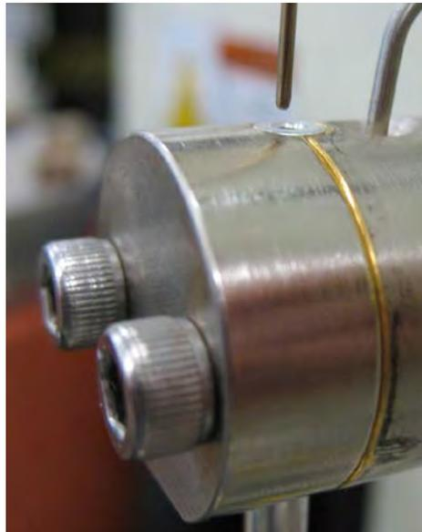
Figure 3-4 – Heater tube holder assembly positioning
