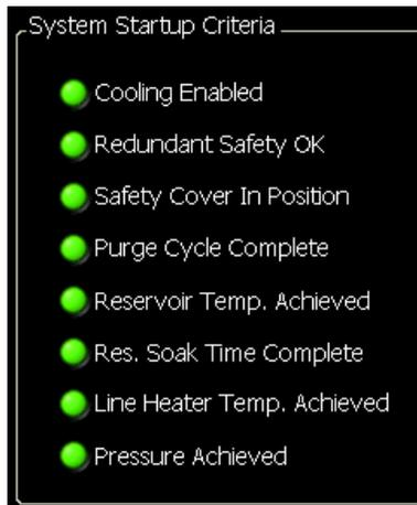
Figure 4-17 – Test startup conditions (based on test configuration)
