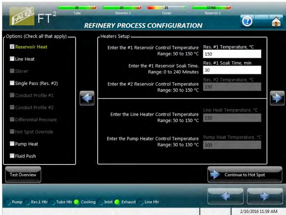
Figure 4-51 – Refinery Process hot spot determination test configuration (optional parameters)
