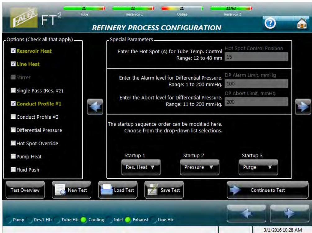
Figure 4-23 – Refinery Process test configuration (special parameter/sequence order)
