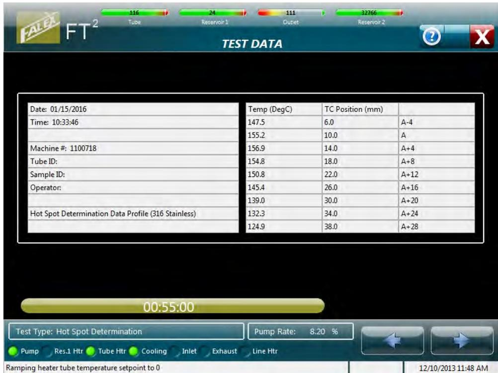
Figure 4-64 – Hot Spot test data display
