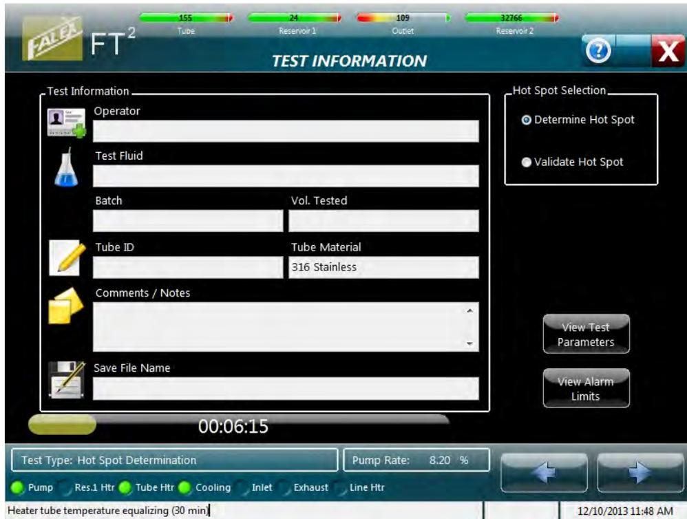
Figure 4-63 – Hot Spot test Information display
