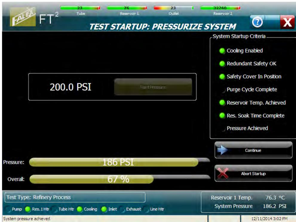
Figure 4-29 – Pressurize System display (with pressurization already initiated)
