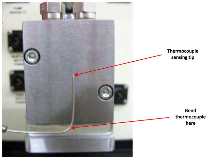
Figure I3 – Thermocouple bends
