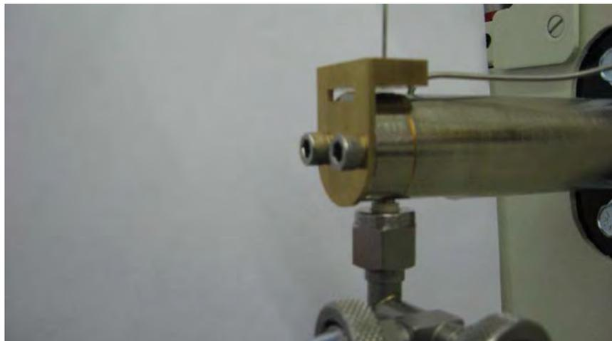
Figure 3-5 – Heater tube thermocouple inserted into heater tube thermocouple guide
