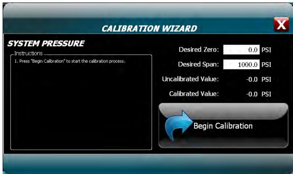
Figure 5-7 – Pressure Calibration Wizard display with Begin button
