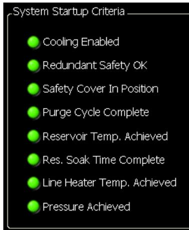
Figure 4-42 – Hot Spot test startup conditions (based on test configuration)
