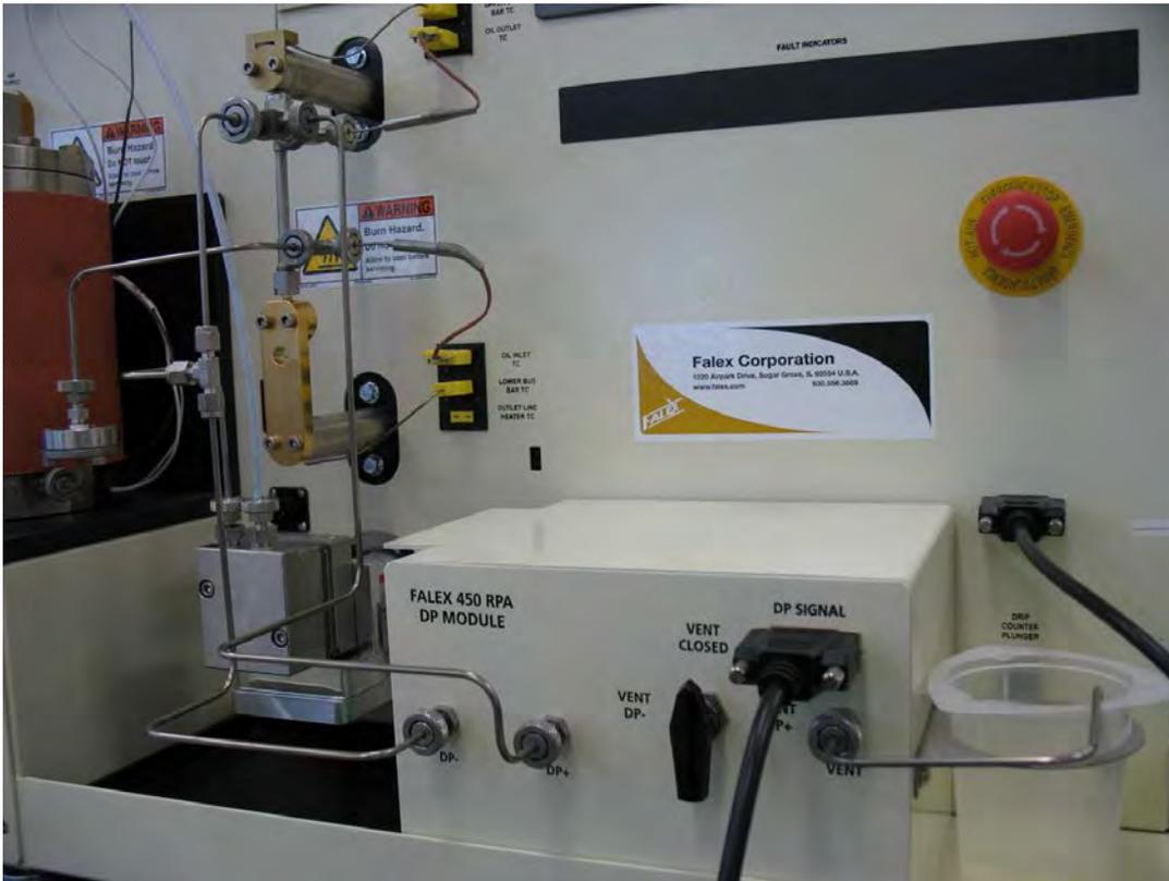
Figure G3 – Differential Pressure (DP) assembly
