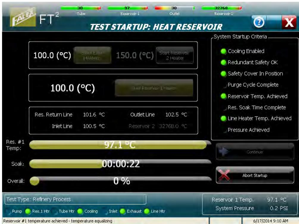
Figure 4-28 – Heat Reservoir display (with heating already initiated and line heaters enabled and already initiated)
