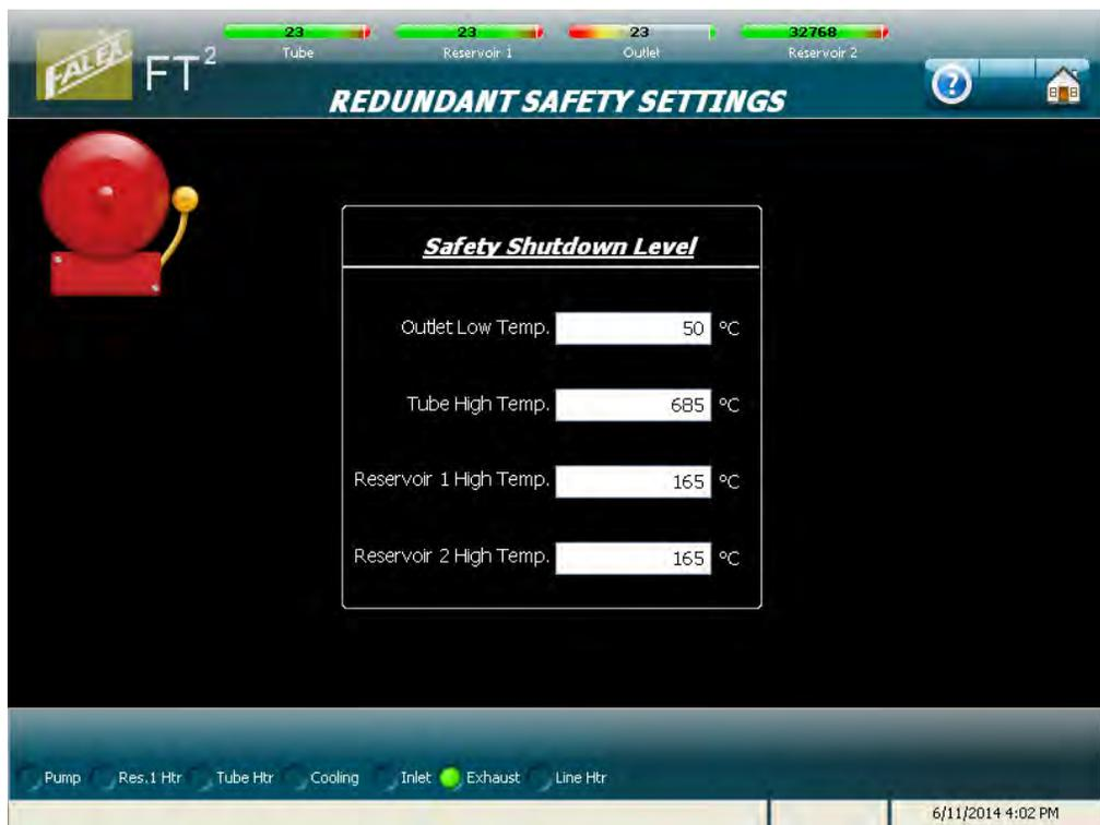
Figure 4-66 – Redundant Safety display (with single pass option enabled)
