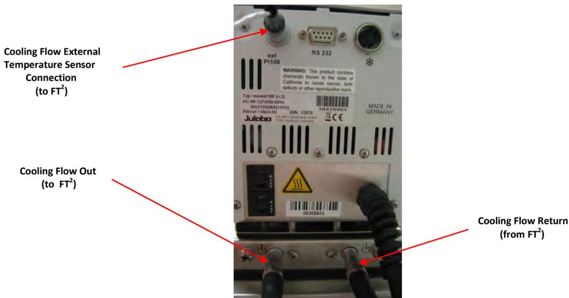
Figure D2 – Circulator Unit (Back)
