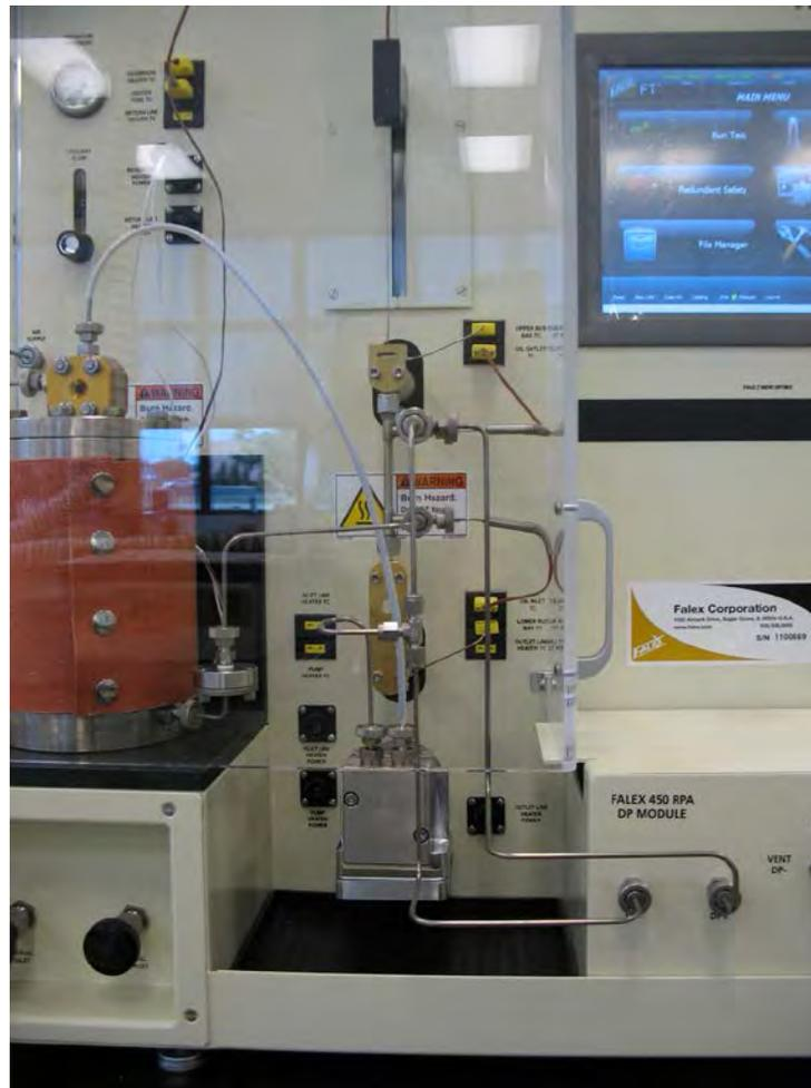
Figure G9 – Assembled differential pressure option (with safety cover)
