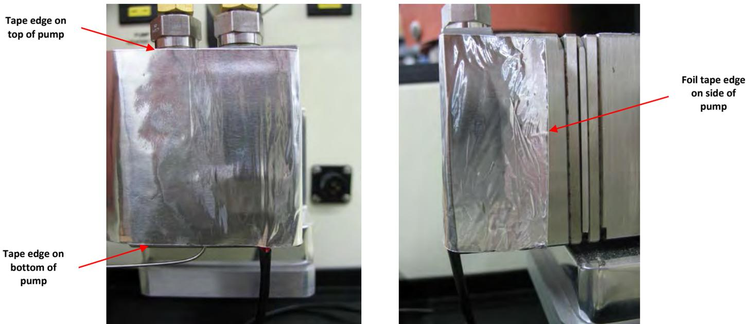
Figure I6 – High temperature foil tape placement
