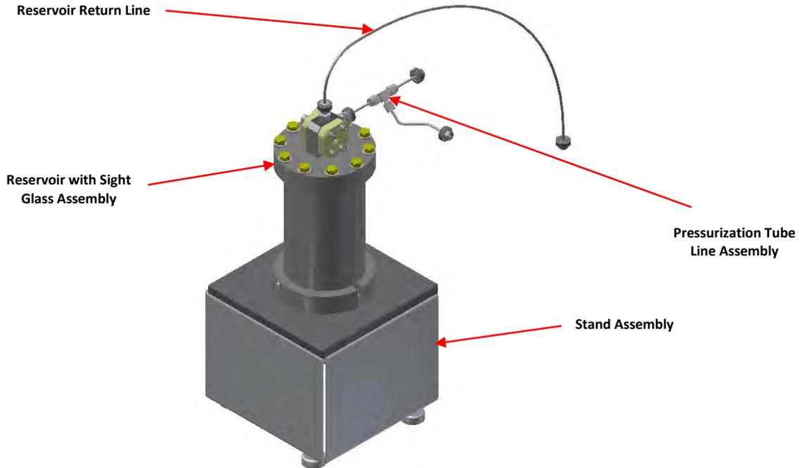
Figure H1 – Single Pass (2<sup>nd</sup> reservoir)
