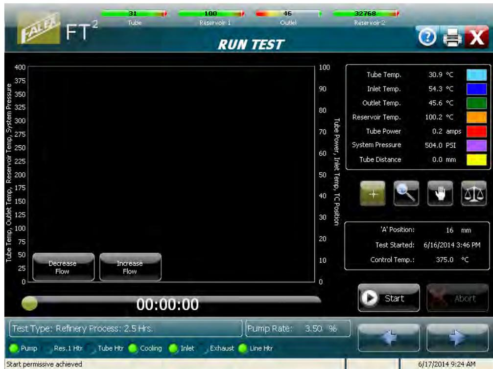
Figure 4-36 – Run Test display
