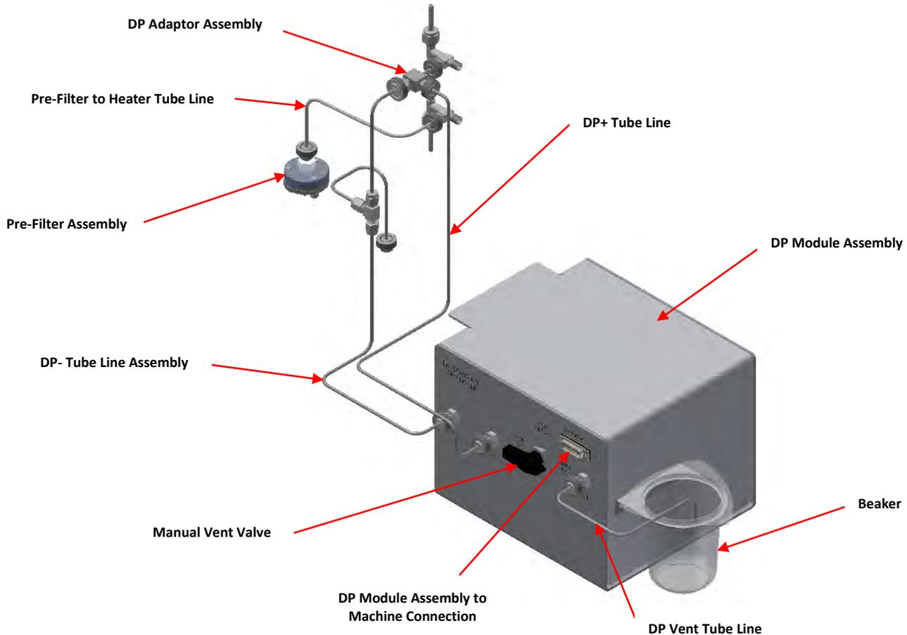
Figure G1 – Differential Pressure (DP) assembly
